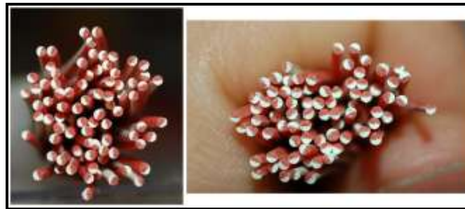
Figure 6. Photos of successfully co-extruded half-moon filaments.
